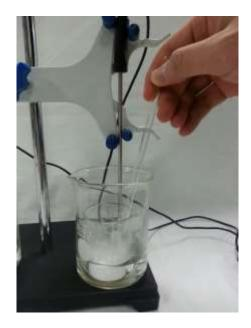
4. After the reactants are well mixed, observe the temperature change in the water in both beakers for 10 minutes.
